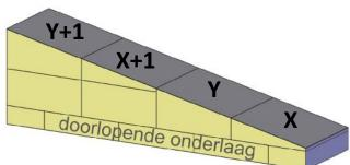
The legend for the installation plans of tapered insulation:
