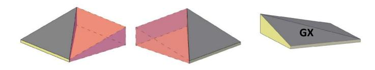
The insulation boards in the form of a ridge are indicated on the installation plan by a sequential letter, which is preceded by a 'G'.
