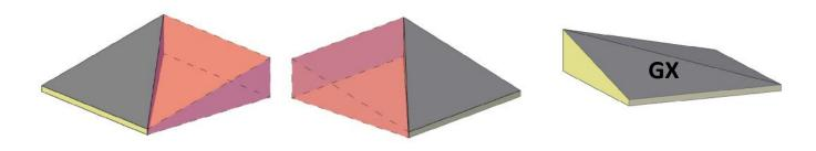
The insulation boards in the form of a ridge are indicated on the installation plan by a sequential letter, which is preceded by a 'G'.
