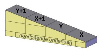
The legend for the installation plans of tapered insulation:
