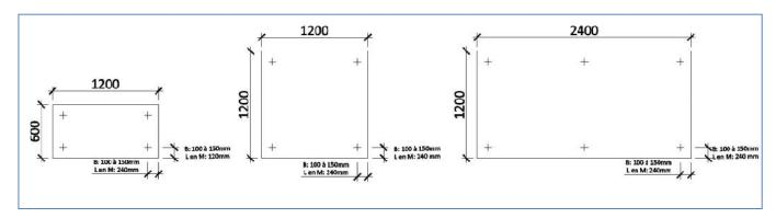
For all zones on the roof surface, the effectively required number of fasteners must be determined in function of the wind load, and in conformity with the regulations of the manufacturer of the roof waterproofing.
